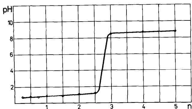
Fig. 2. The pH dependence on the molar ratio \text{Na}_2\text{TeO}_3 \cdot \text{Hg}(\text{NO}_3)_2 .
